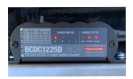
Start the engine and after a short time the vehicle light should come on and the stage light will either be solid on or flashing depending on the state of charge of the battery. This can be seen in the image.
