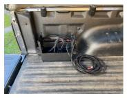
Mount box into position by re installing the bolts removed, 2x bolts from tie down and 2x bolts on bracket at rear of tub. Next mark and drill 2x extra holes in floor of tub and use bolts and nuts supplied in kit to secure extra 2 bolts in tub floor. Tighten all 6 bolts securing box into position.
