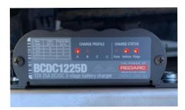
Start the engine and after a short time the vehicle light should come on and the stage light will either be solid on or flashing depending on the state of charge of the battery. This can be seen in the photo.
