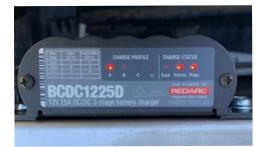
Start the engine and after a short time the vehicle light should come on and the stage light will either be solid on or flashing depending on the state of charge of the battery.
