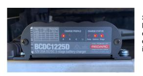
Start the engine and after a short time the vehicle light should come on and then the stage light will either be solid on or flashing depending on the state of charge of the battery. This can be seen in the image.
