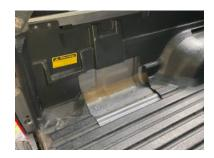
In models with a tub liner - sit the box into position as shown in the TLR instruction manual and trace around box to prepare for cutting the liner to make way for the battery box. To aid in this step please view one of our installation videos on our YouTube channel, here is a link to one of them Installation video
