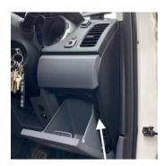
This image shows the tab to push up which will allow the storage tray to come out and expose the fuse box
