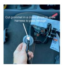
battery continue to route toward main battery. The one labelled ignition route into cab through grommet under passenger seat.
