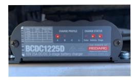
Start the engine and after a short time the vehicle light should come on and the stage light will either be solid on or flashing depending on the state of charge of the battery.
