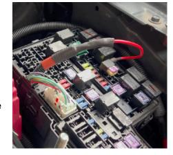
Replace this fuse with the 'add a fuse', fuse holder found in the kit and plug the fuse holder lead into the small harness labeled ignition. Use the supplied heat shrink to cover the join and shrink down over join.
