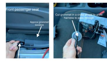
The next step is to run the small ignition wire to the car fuse box under the steering wheel. First we will need to remove the passenger side trims.
