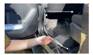
Follow Ford harness toward fuse box under the dash. Securing the harness to existing cables with cable ties supplied.
