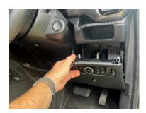
Access the fuse box below the steering wheel by removing the panel as shown in the image.
