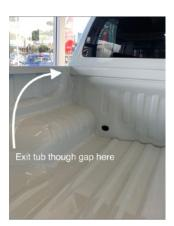
Start by routing cables out of the tub by exiting through the tub close to the back of the cab. This step may change depending on whether the tub has a canopy or hard cover. If this section of the tray is not accessible then a cable gland is supplied to allow cable to be routed out of tub.
