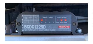
Start the engine and after a short time the vehicle light will come on and the stage light will either be solid on or flashing depending on the state of charge of the battery. This can be seen in the image.
