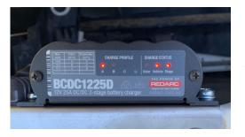
Start the engine and after a short time the vehicle light should come on and the stage light will either be solid on or flashing depending on the state of charge of the battery. This can be seen in the image.
