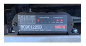
Start the engine and after a short time the vehicle light should come on and then the stage light will either be solid on or flashing depending on the state of charge of the battery. This can be seen in the image.
