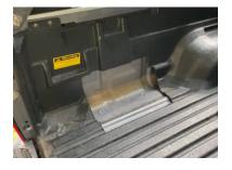
The next step will be to mark (trace outline) where the box is going to be installed, lining up with 2x factory bolts in the tub floor and then to cut out the tub liner to allow the box to sit flush into position.
